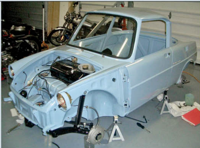
Simple rubber-filled torsion tube suspension was in great shape. Re-assembly of bare shell meant that fit after painting was guaranteed
