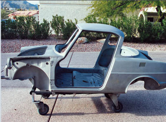
It's a unibody, but not much of one; aside from fenders, almost everything comes off. Low-pressure iron oxide blasting used for stripping
