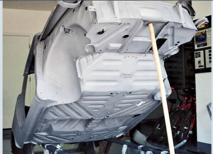
No rotisserie needed when a body shell is around 150 pounds; owner was able to tilt it by hand and prop it up for undercarriage work
