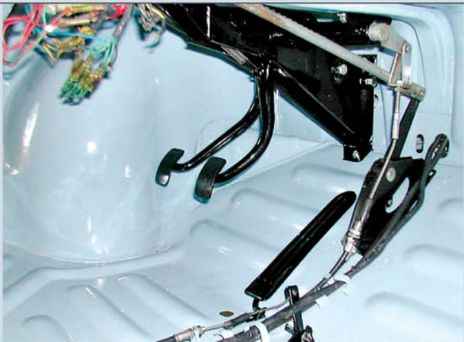
Interior black is straight black toner, sprayed on. Interior sheetmetal got the same priming and painting as exterior, minus polishing
